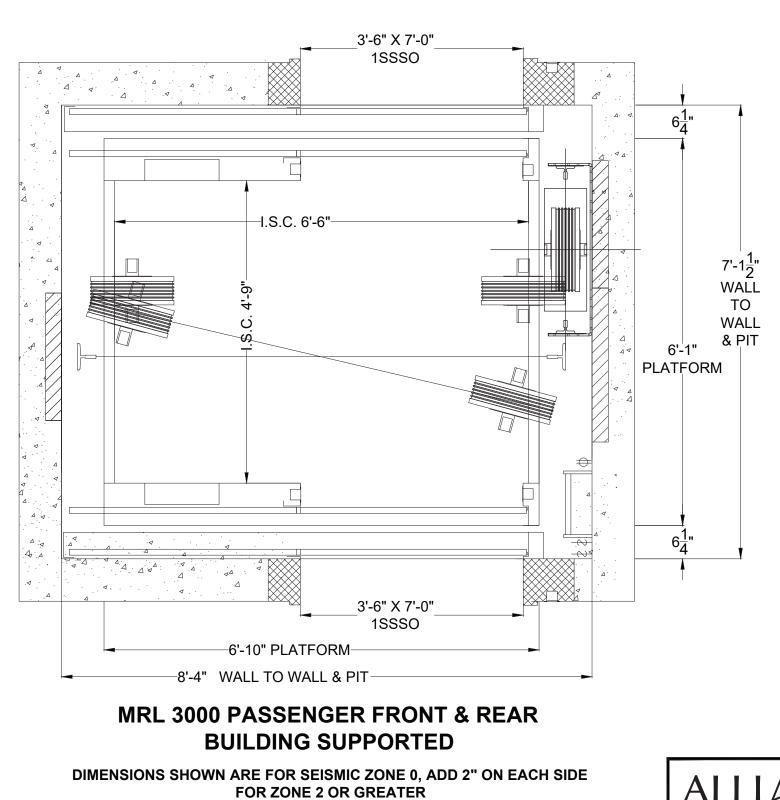
DIMENSIONS SHOWN ARE FOR SEISMIC ZONE 0, ADD 2" ON EACH SIDE FOR ZONE 2 OR GREATER
